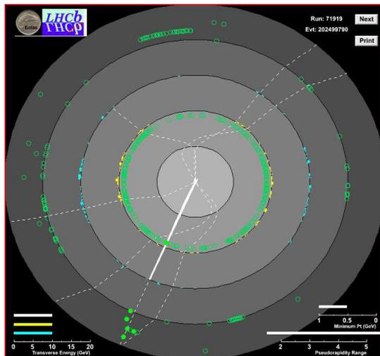
Figure 2: LHCb’s first  $W^+ \rightarrow \mu^+\nu$  candidate, shown in a ‘ $z - \phi$  view’ of the detector, with the Vertex Locator at the centre and muon stations at the periphery of the display. The white thick straight line represents a high  $p_T$  track ( $p_T = 35.4 \text{ GeV}$ ) with hits in the muon chambers, while the curved dotted lines are accompanying soft tracks.
