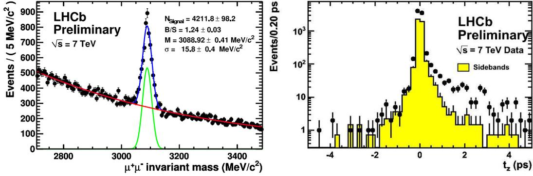
Figure 5: Left: Dimuon invariant mass distribution showing the  $J/\psi \rightarrow \mu^+\mu^-$  signal in  $\sim 14 \text{ nb}^{-1}$  of data at  $\sqrt{s} = 7 \text{ TeV}$ . Right: Pseudo-proper time distribution of the  $J/\psi$  candidates in the signal window (black points) and in the sidebands (yellow histogram). The difference between the two distributions corresponds to signal  $J/\psi$  and displays a tail at large proper time indicative of  $b \rightarrow J/\psi X$  production.
