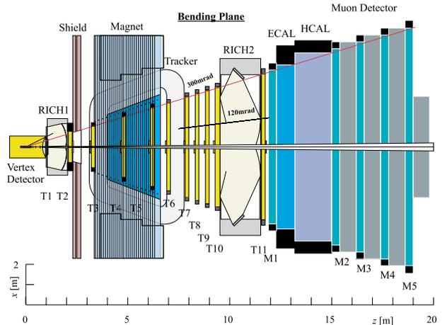
Figure 3: Top View of the LHCb detector.
