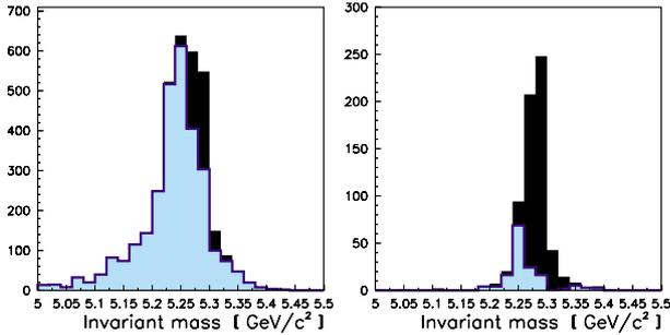
Figure 4: Simulated invariant mass distribution for  $B_s \rightarrow D_s \pi$  reconstructed with the LHCb spectrometer without applying particle identification (left) and with information from the RICH detectors (right). Background contribution is indicated by the lighter colour.
