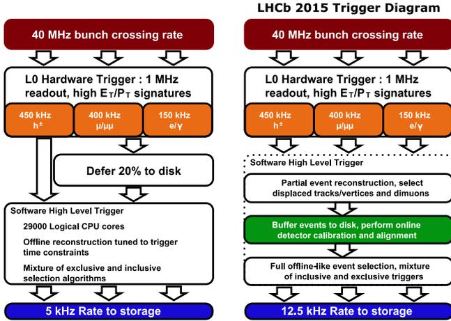
Fig. 1. Schematic diagram of the LHCb trigger data-flow in Run I data taking (left) compared to the proposed data-flow in Run II (right).
