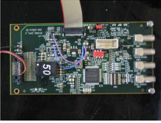
Figure 2: Front-end electronics to read out the MPPCs.
