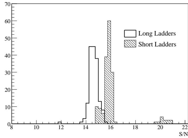
Figure 3: Measured S/N of the Inner Tracker ladders.
