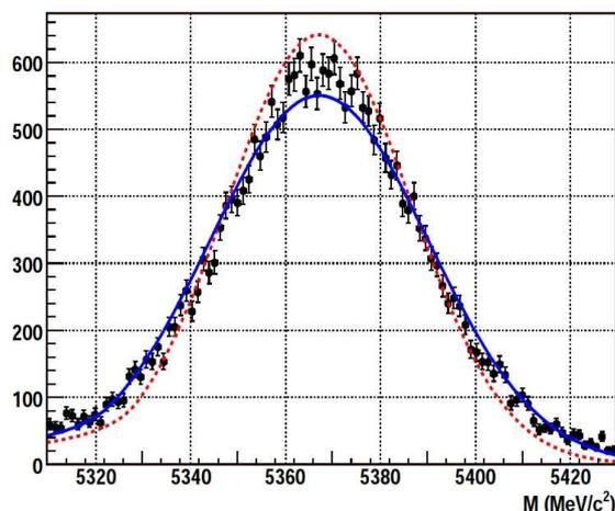
**Figure 3:** Invariant mass distributions for  $B_s^0 \rightarrow K^+ K^-$  with a correction for the kaon identification cut effect (solid curve) and without correction (dashed curve). Points with error bars represent  $B_s^0 \rightarrow \mu^+ \mu^-$  invariant mass distribution.
