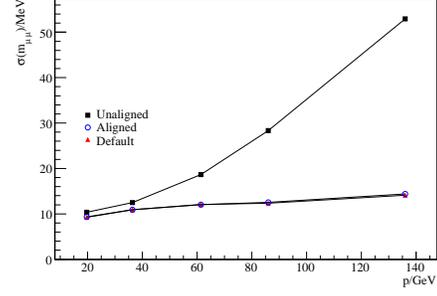
Fig. 11.  $J/\psi$  mass resolution versus  $p/\text{GeV}$ .
