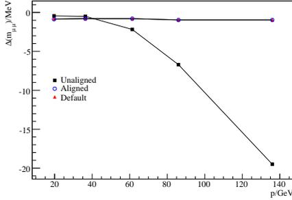
Fig. 10. Bias on the  $J/\psi$  mass versus  $p/\text{GeV}$ .
