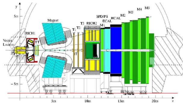
Fig. 1. Side view of the LHCb detector.
