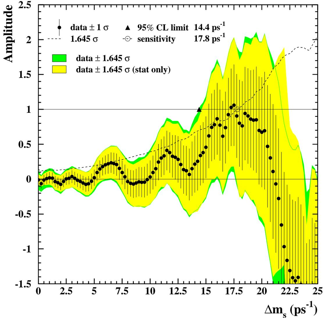
Figure 2: Combined measurements of the  $B_s^0$  oscillation amplitude as a function of  $\Delta m_s$ , including all results published by November 2003. The measurements are dominated by statistical uncertainties. Neighboring points are statistically correlated.
