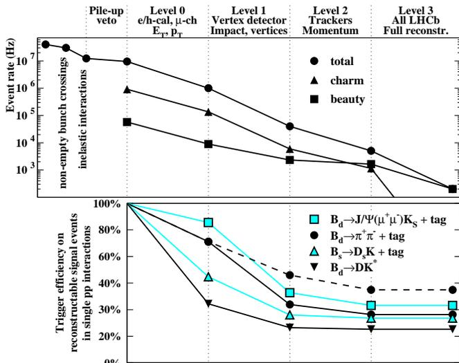
Figure 3: Summary of the LHCb trigger performance, with event rates (top) and efficiencies for signal events usable in the offline analysis (bottom) after each trigger level. The dashed line shows the effect of using Level-0 information for the Level-1 trigger.<sup>6</sup>
