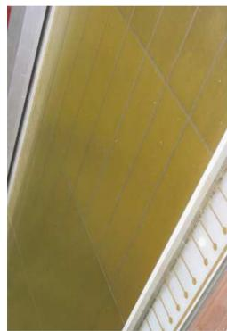
Muon MWPC prototype
