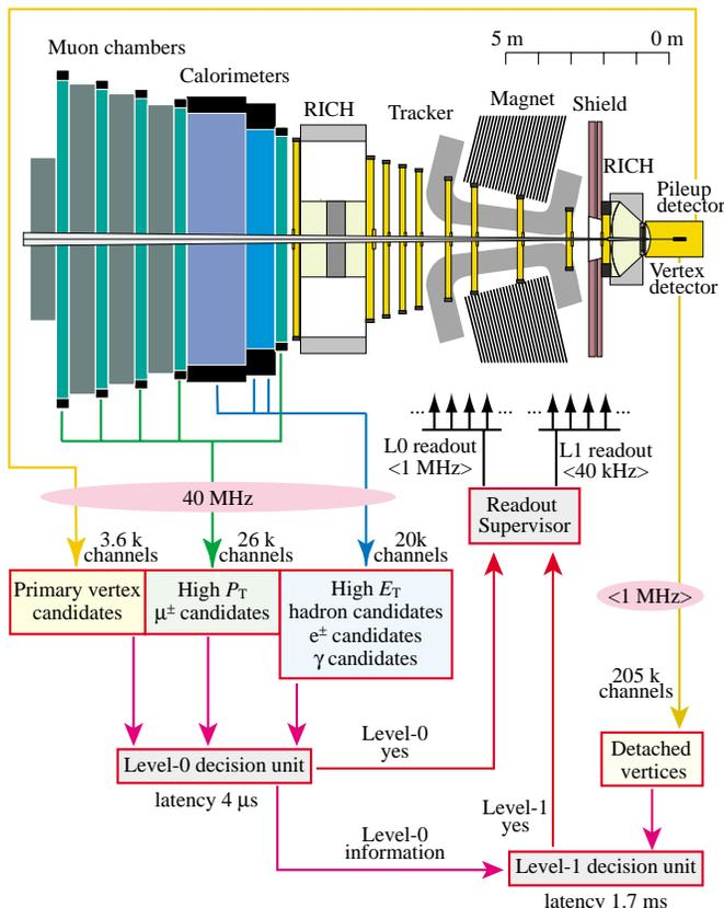
Figure 1: Side view of the LHCb detector (in the non-bending plane) and overall scheme of the first two trigger levels.
