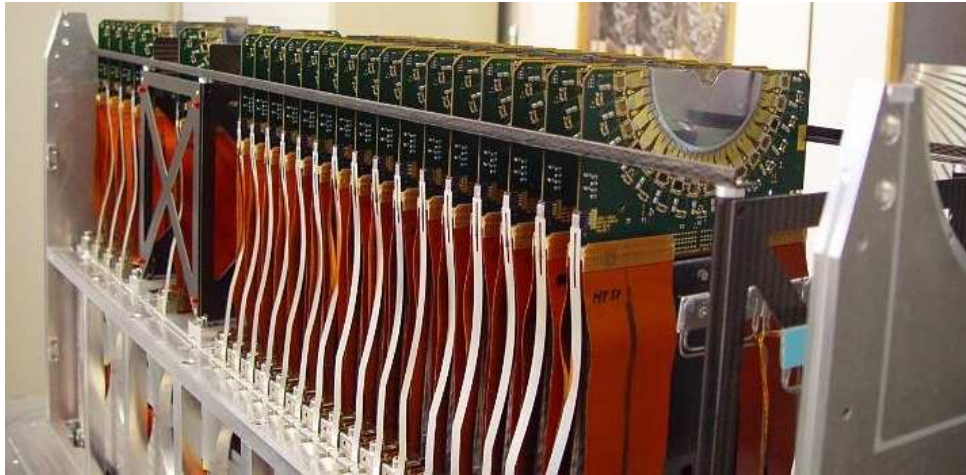
Figure 2: 21 VELO modules (holding the half-disk silicon sensors) installed on their support and forming half of the VELO detector.
