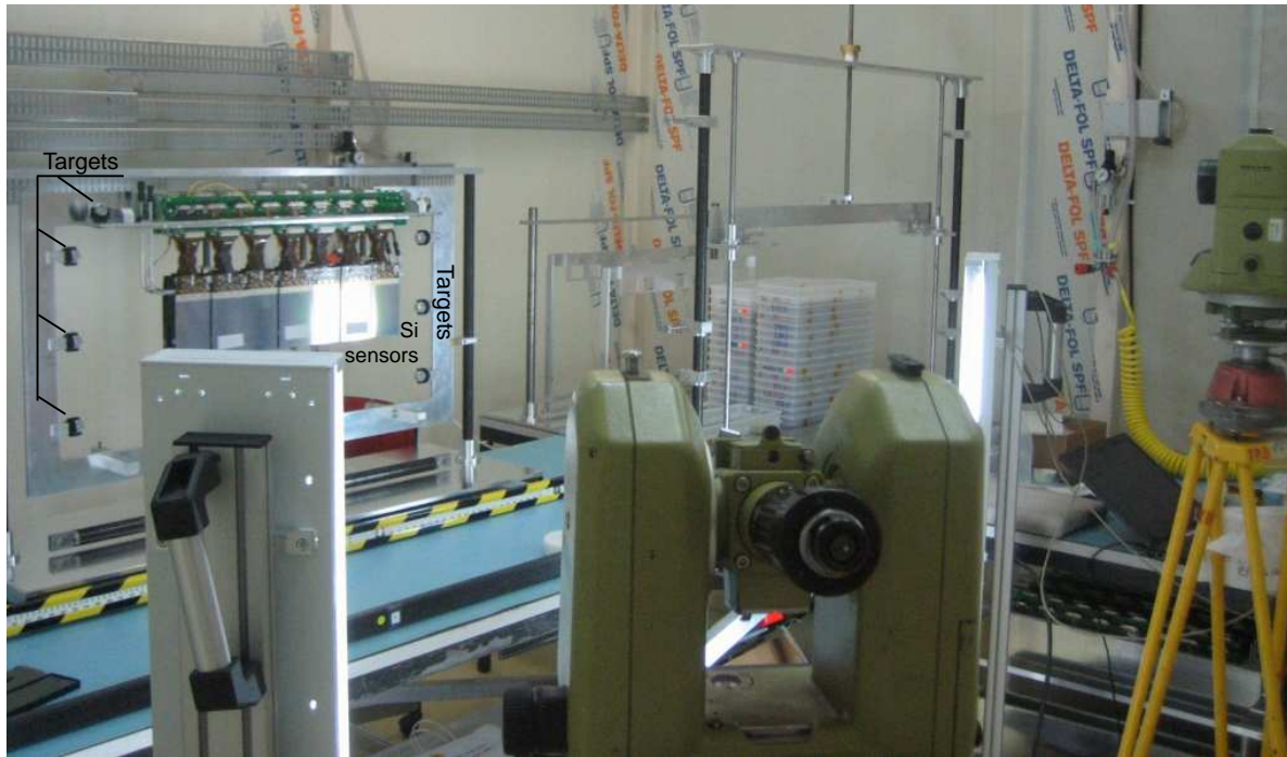
Figure 5: IT detector survey using two theodolites. On the left, four layers of silicon sensors attached to a box cover are hanging on a revolving frame on which targets have been placed.
