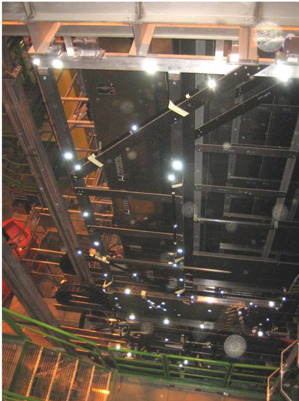
Figure 4: Support frames of three half-stations of the Inner Tracker installed in the pit (behind each other). Reflecting targets used for the photogrammetry can be seen on the first support frame (IT1).
